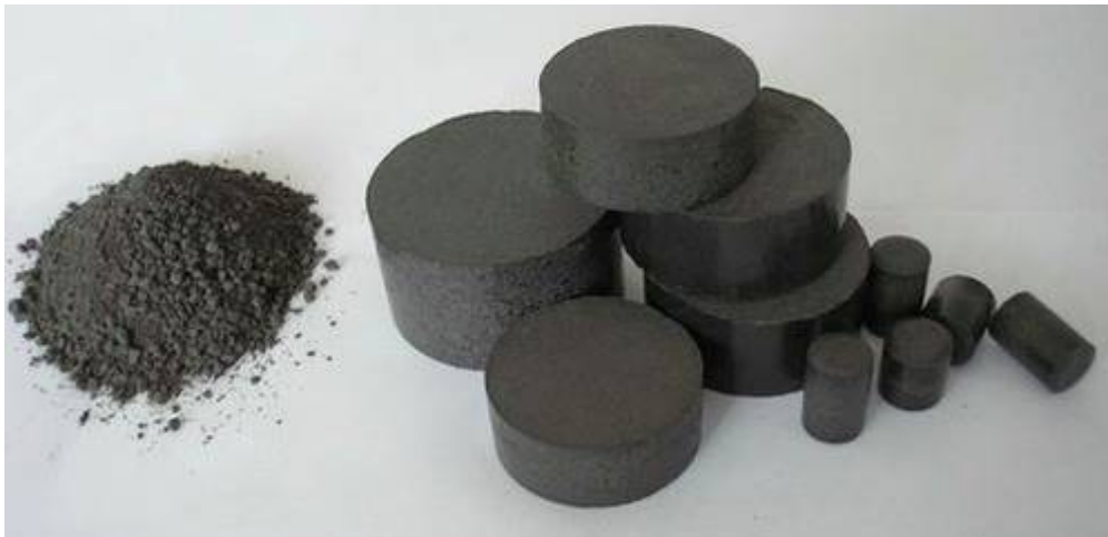
Figure 15-1 Granular (left) and pelletized (right) epoxy molding compound 2
