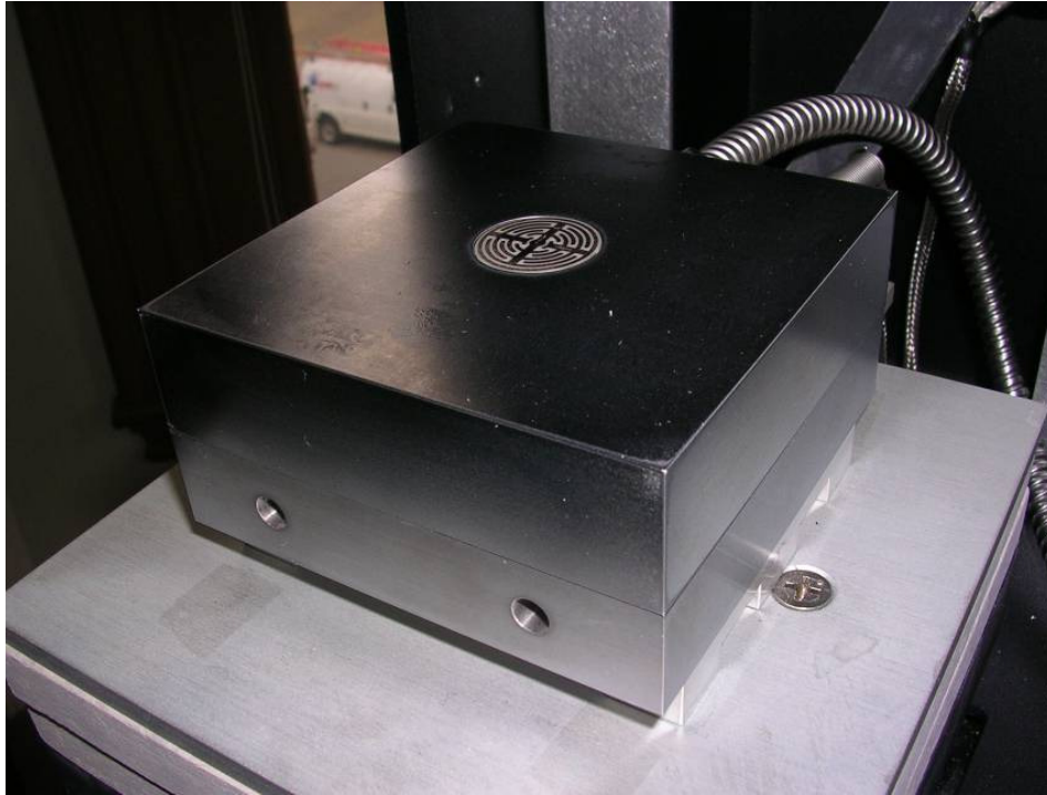
Figure 17-1 Ceramiccomb-1" reusable sensor embedded in press platen
